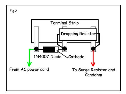
Step 6. Determine the value of the dropping resistor. If you are leaving the 130 ohm sand resistor in place, use gator wires to connect a 50 ohm, 5 watt resistor to the cathode end of the silicon diode and the other to the 130 ohm resistor. Connect your multimeter to pins 1 and 7 of the 1L6 tube (Fig. 5) and read the DC voltage as you bring the voltage up to 120 VAC on a Variac. Don't let the filament voltage go over 1.4 volts DC.
