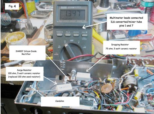
If you are replacing the 130 ohm sand resistor with a resistor of a different value, then you may need to experiment with various combinations of dropping and surge resistor values.
