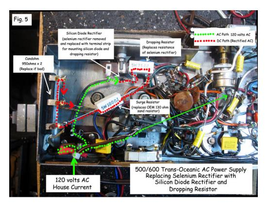
The values shown above are for the specific G500 Trans-Oceanic used as an example. Your values will vary, depending on the condition of your radio and whether you are just replacing the selenium rectifier, or other components in the power supply as well.
