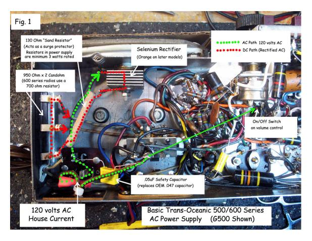
120 volt AC current enters the radio through the power cord. One leg goes to the on/off switch located on the volume control. The other leg goes to the anode terminal on the selenium rectifier. The selenium rectifier removes, or blocks, one half of the AC sine wave, converting AC to DC current, although not a perfect DC current. The electrolytic capacitors filter this rippling DC current to even it out.
