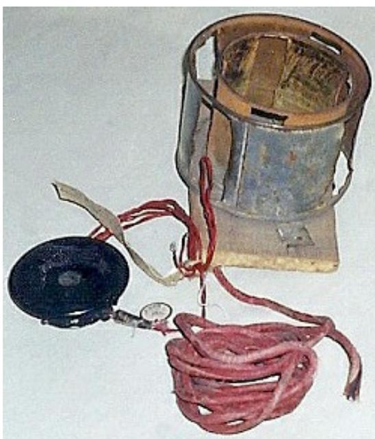
Part of crystal receiver #4 with missing detector and coil. Particularly of interest is the tuning condenser made from two tin cans with cut-out slots. Though not identical to the 'Tin can' radio of Chapter 207, it was also based on the use of two empty tin food cans.
