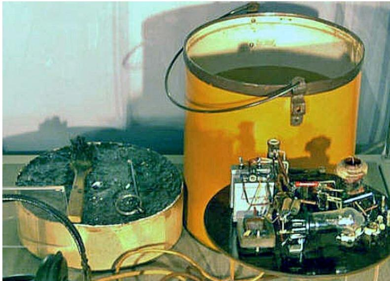
Replica of the 'Pail receiver' constructed in the 1960s.
