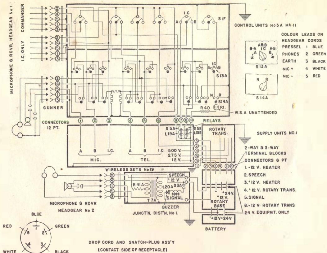
FIG. 8—WIRING LAYOUT OF A CANADIAN INFANTRY TANK MK111\*\*\* INSTALLATION
