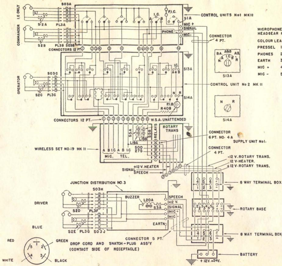
FIG. 9—WIRING LAYOUT OF A U. S. MEDIUM TANK M-4
