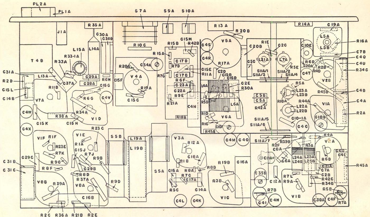
FIG. 6—UNDERNEATH PLAN OF CHASSIS
