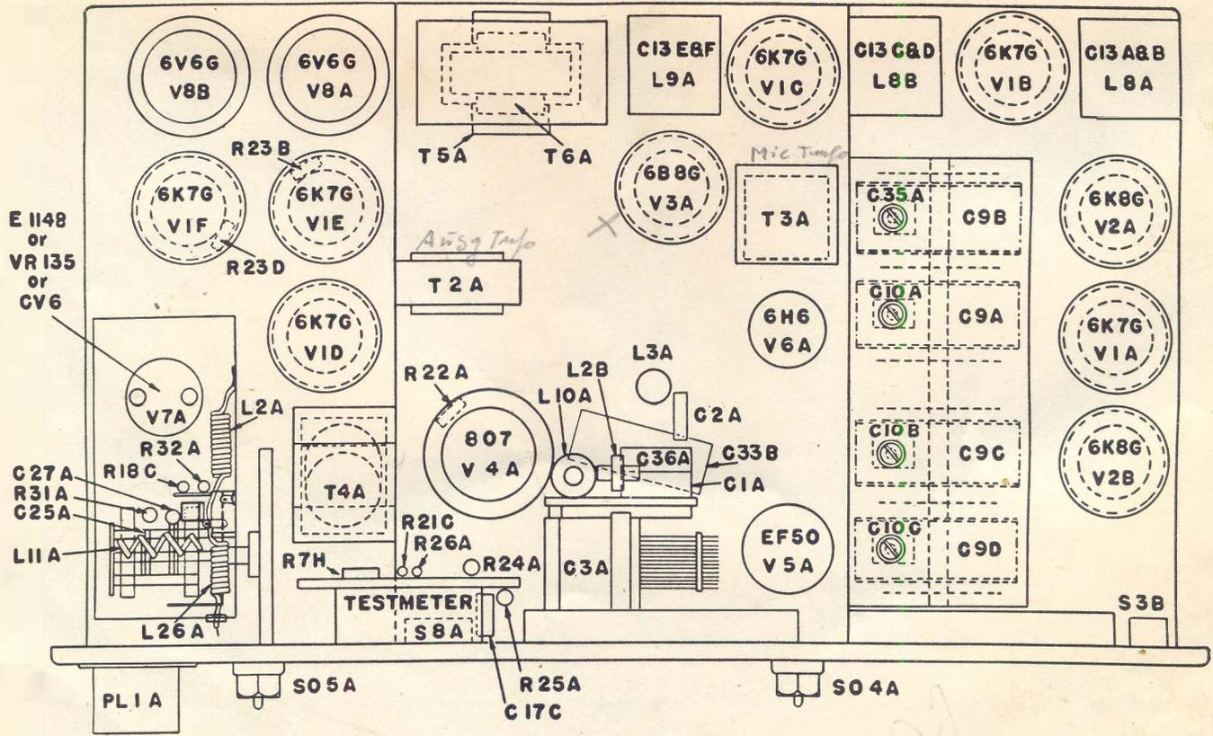
FIG. 5—TOP PLAN OF CHASSIS
