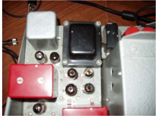
Leary's audio section, 6C4, 6BA6, 12AX7 and 6AQ5 like Collins 75A-4 (don't ask)
