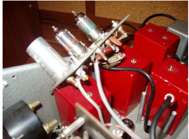
Product detector that sets on top of spacer studs over the 2nd conversion section on chassis
