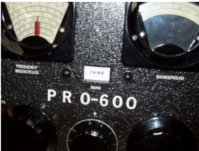
Band in use plate painted by Cecil and the engravings were filled in using a black lacquer stick (was brass and couldn't read it)
