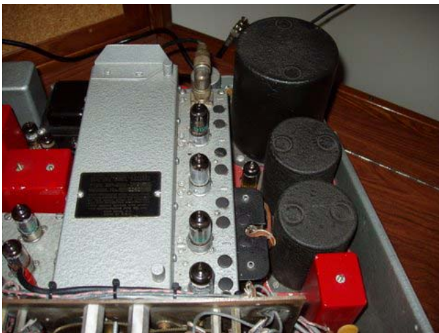
RF Deck, using a 6BZ6 1st rf amp tube
