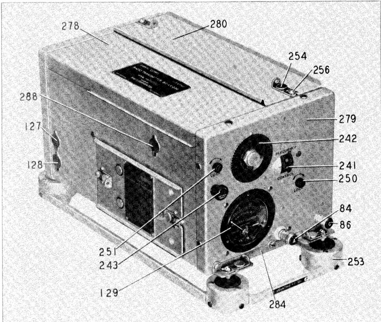
FIGURE 4—RADIO TRANSMITTER BC-AS-230 WITH COIL SET C-435 IN PLACE
