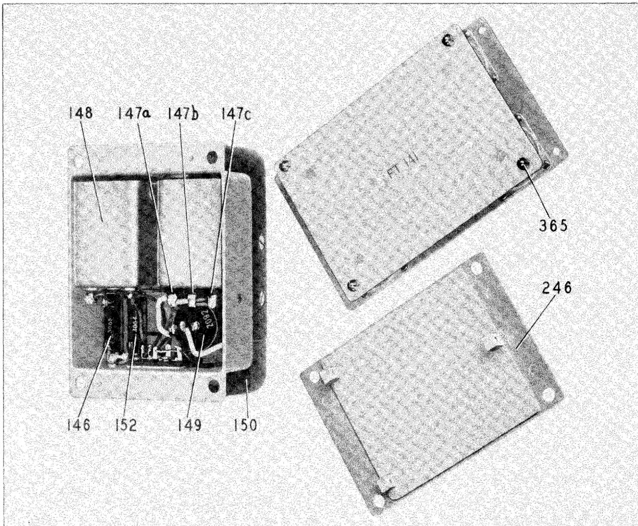
FIGURE 8—DYNAMOTOR UNIT BD-AS-83, BOTTOM VIEW
