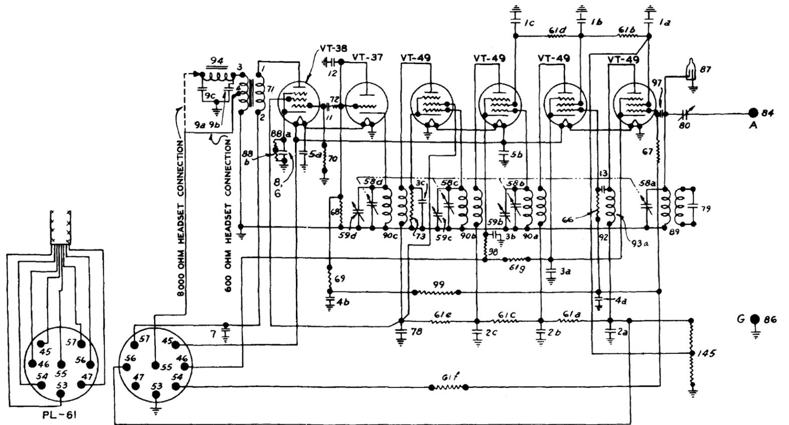
FIGURE 19-RADIO SET SCR-AS-183, SCHEMATIC CIRCUIT DIAGRAM
