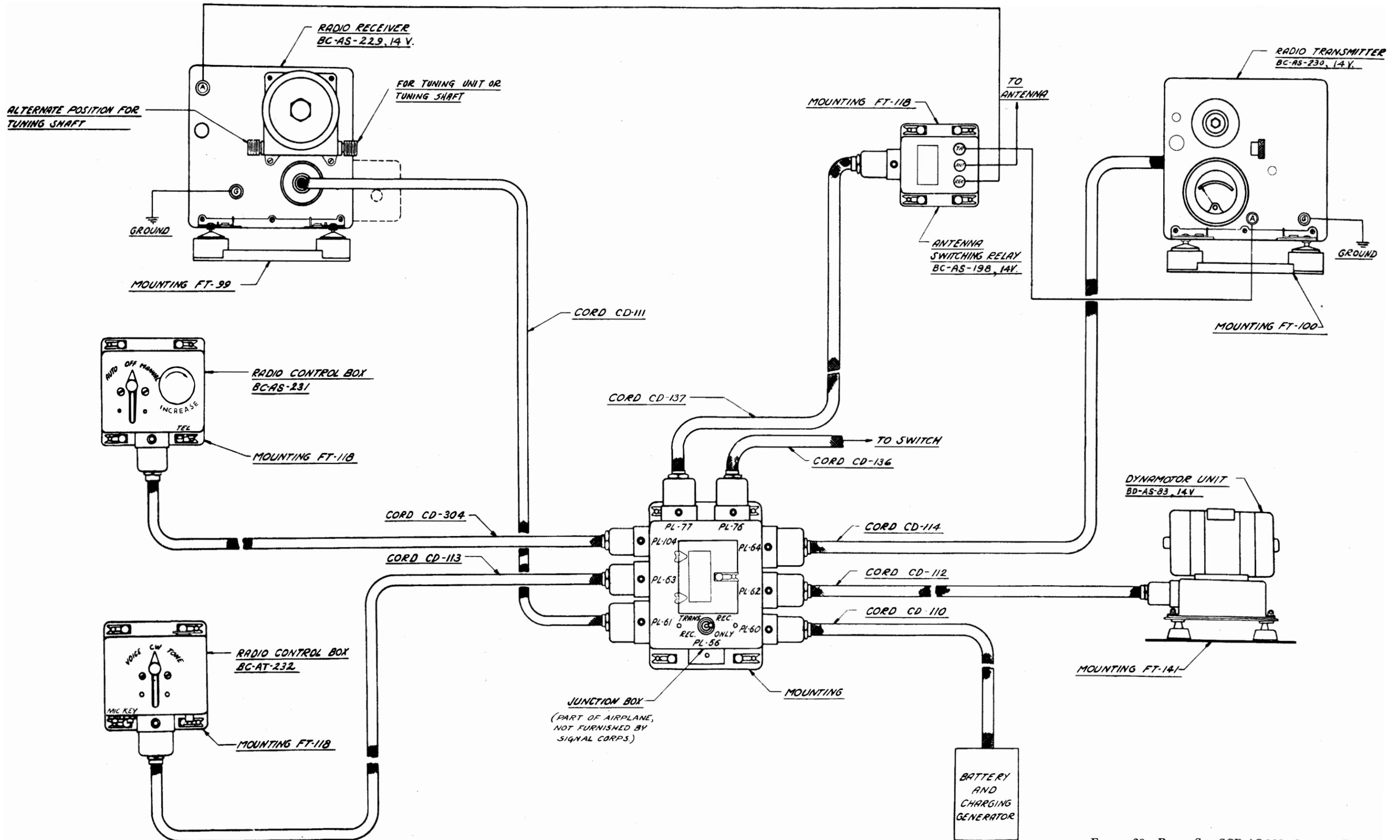
FIGURE 20—RADIO SET SCR-AS-183, CORDING DIAGRAM
