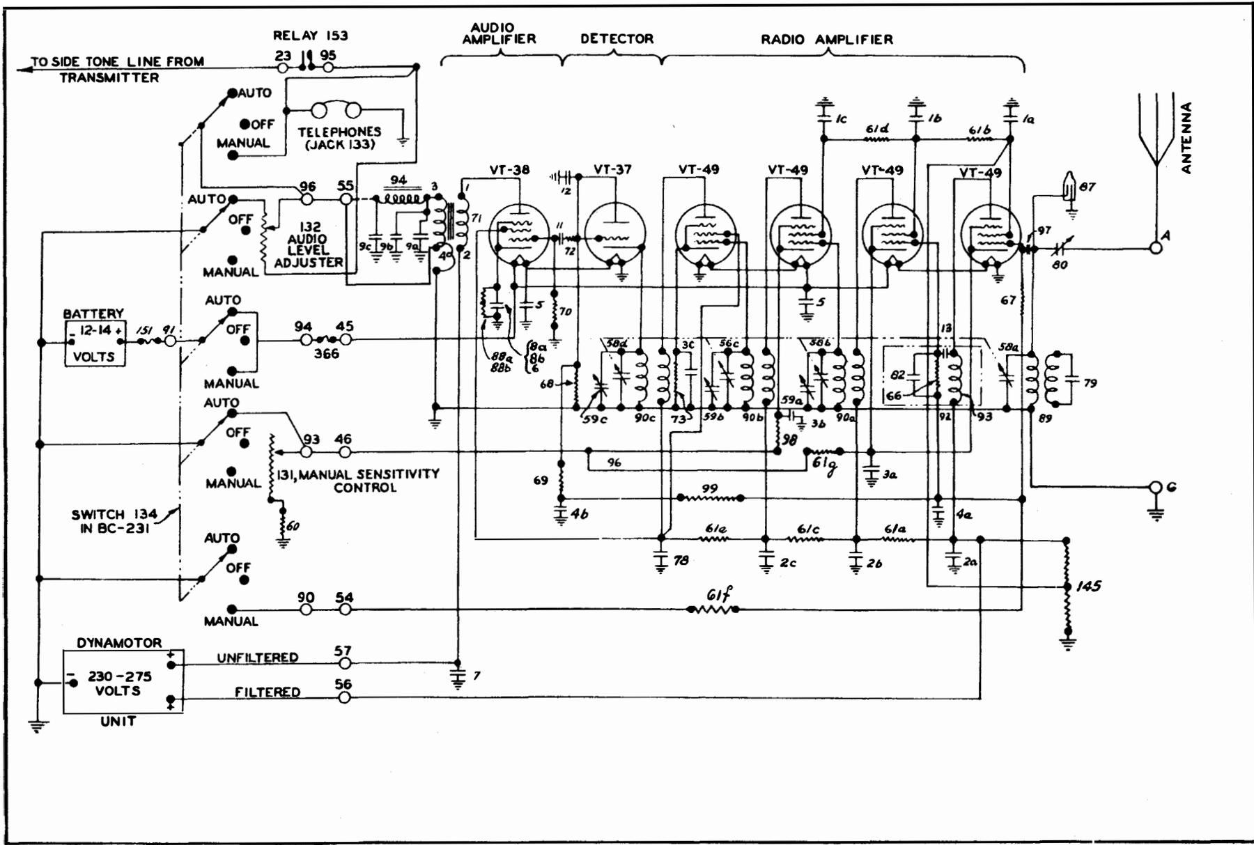
FIGURE 17—RADIO RECEIVER BC-AS-229, FUNCTIONAL DIAGRAM
