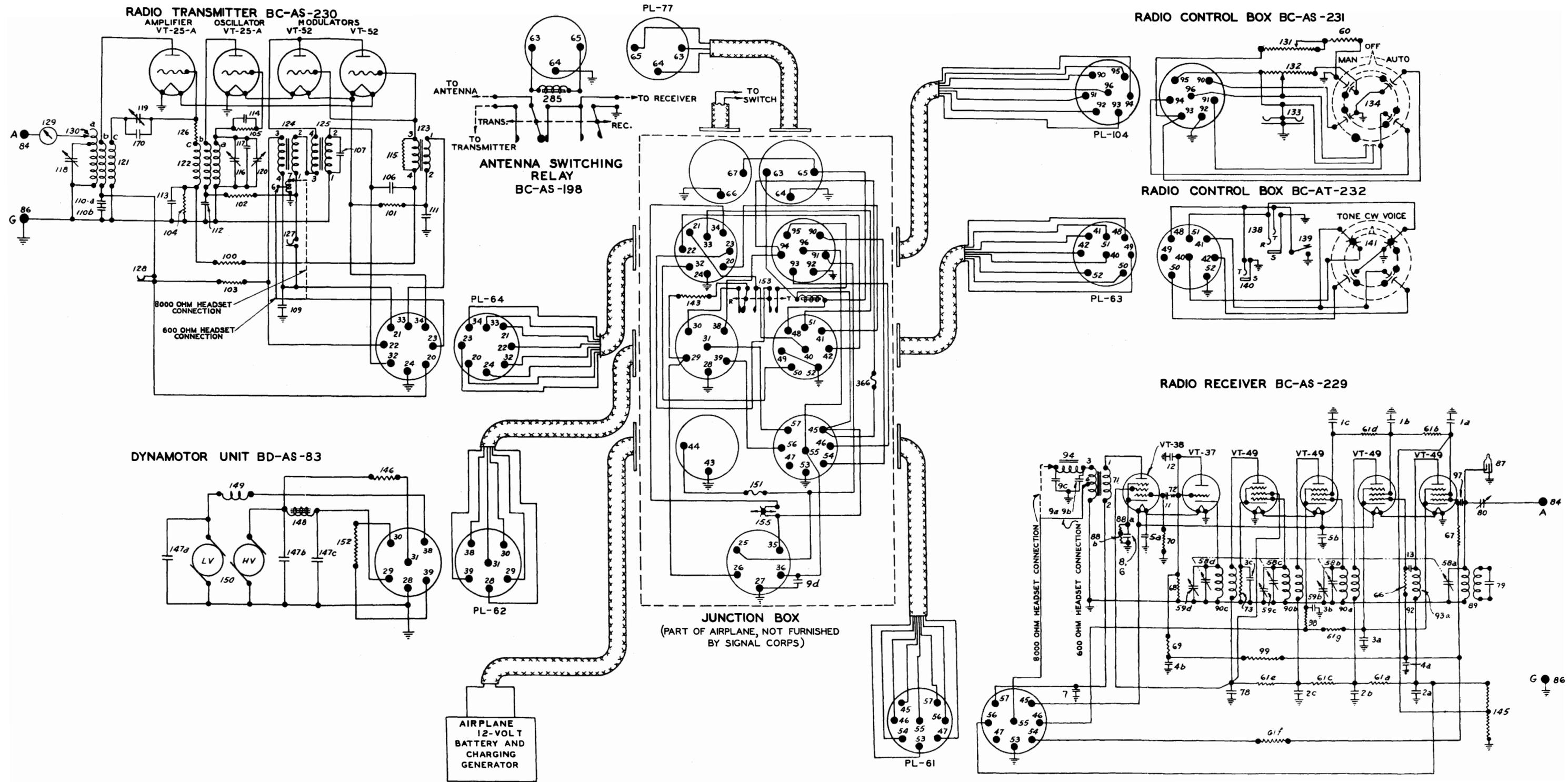
FIGURE 19-RADIO SET SCR-AS-183, SCHEMATIC CIRCUIT DIAGRAM
