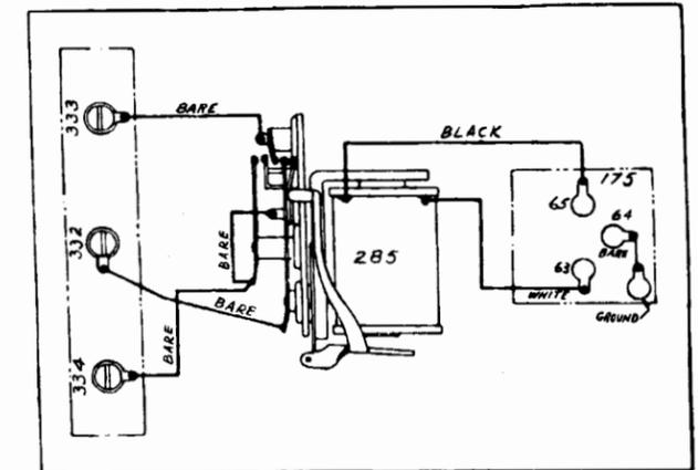
FIGURE 21—COMPONENTS OF RADIO SET SCR-AS-183, PRACTICAL WIRING DIAGRAM
