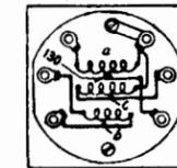
AMPLIFIER COIL ASSEMBLY FOR COIL SETS C-431, C-432, C-433, C-434 & C-435 UNSHIELDED
