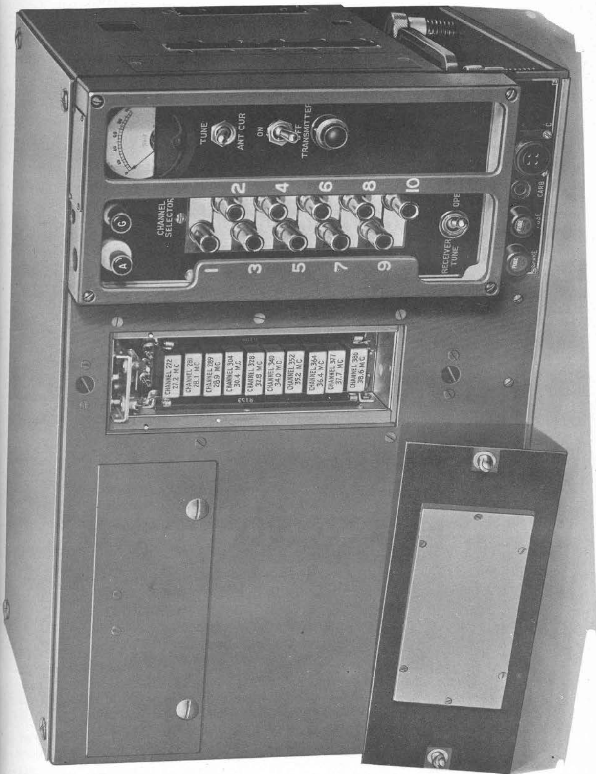
Fig. 12. Radio Transmitter BC-684-A: Front View with Crystal Compartment Open
