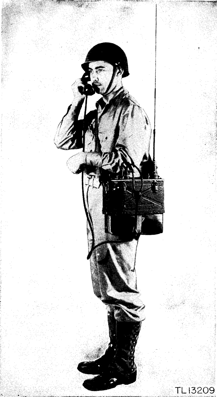
Figure 19. Radio Set SCR-300-A, lightweight installation.
