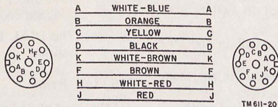
Figure 67. Cable Assembly CX-1212/U, schematic diagram.
