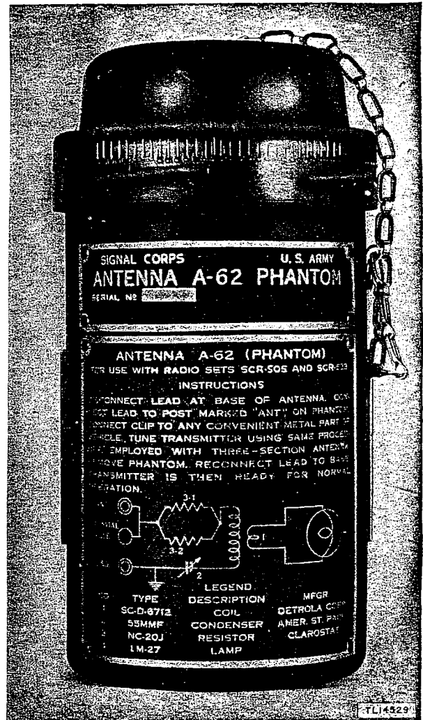
Figure 25. Antenna A-62 (Phantom), showing nameplate and circuit label.
