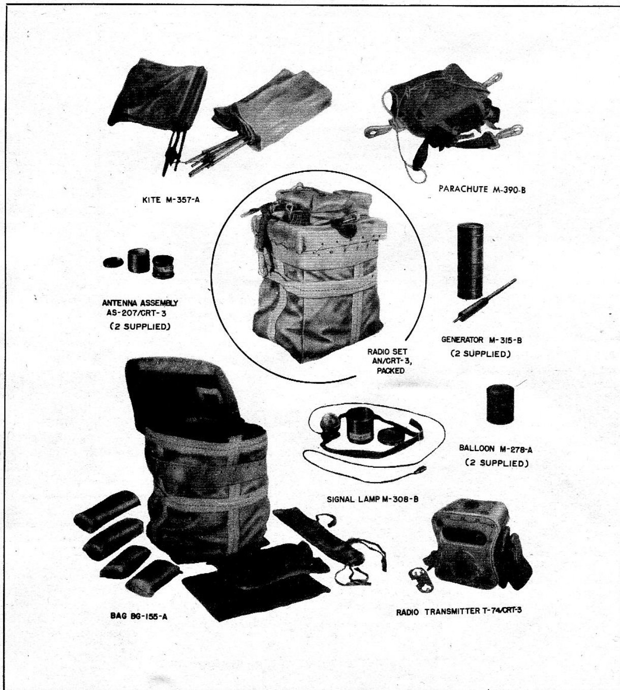
Figure 1-1. Radio Set AN/CRT-3—Major Assemblies
