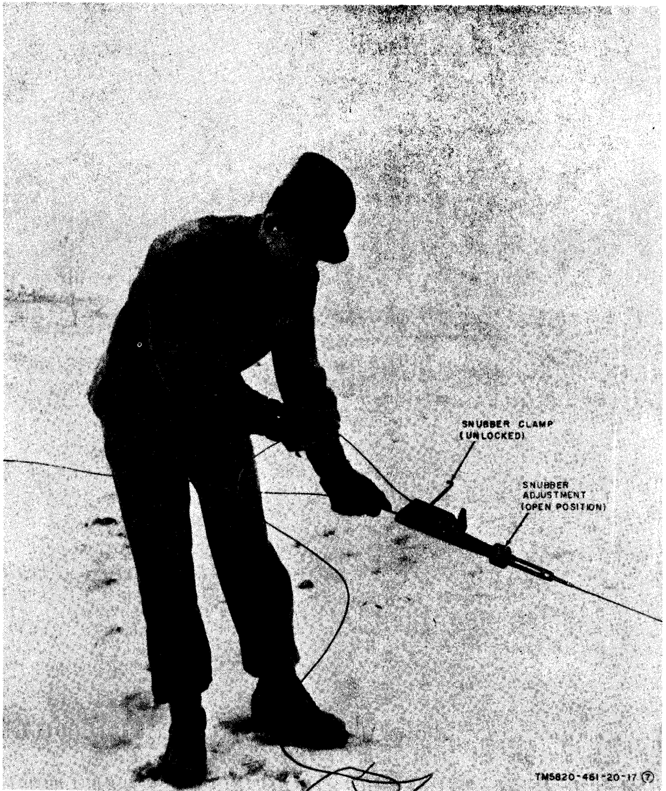
Figure 2-17⑦. Erection of launcher (part 7 of 9).
