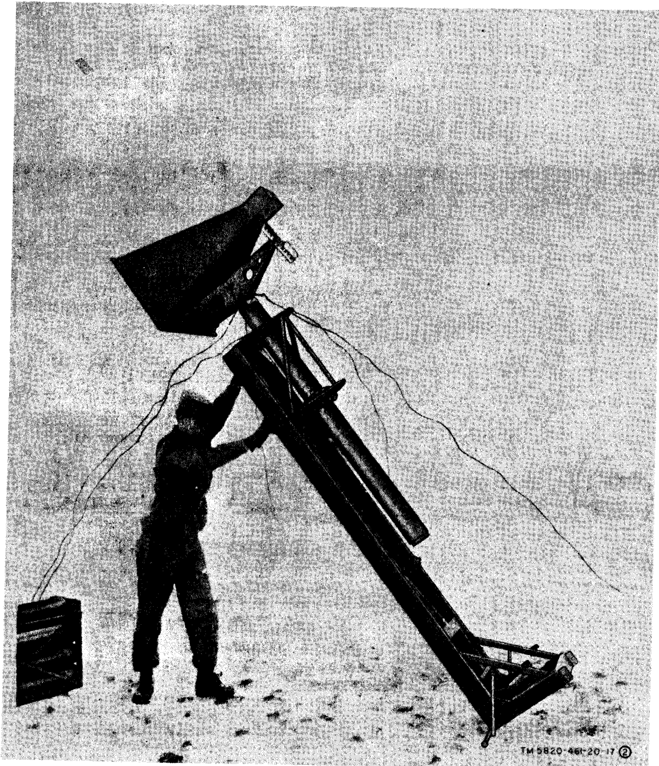
Figure 2-17 Ⓢ. Erection of launcher (part 2 of 9).
