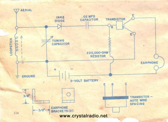
Ground Tuning Capacitor Loopstick Crystal Tie Point Diode Aerial Capacitor Transistor sistor EB C Earphone MECHANIX ILLUSTRATED **Batteries Transistor**
