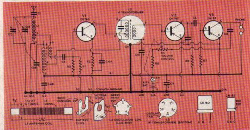
TO IDENTIFY LEADS of coils and transistors, hold them in the positions shown directly above and compare with the drawings Kex letters on the marked in the pictorial diagrams on page 198.
