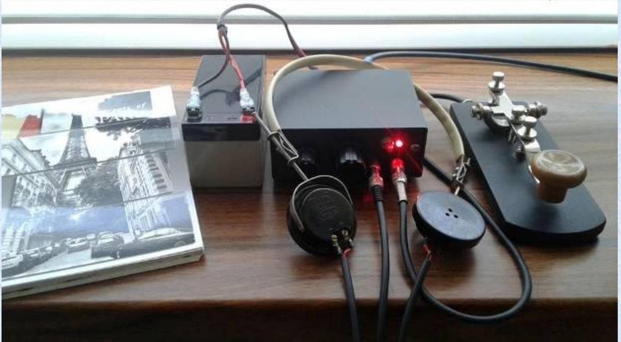
This is basically a crystal receiver with BFO. Not so sensitive but capable for making QSO, proven already. About 20 stations are in my log using this trcvr. Without headphones I can use it as TX only, but plugging in the headphones its resistance triggers the BFO. Quite selective, but since we knew selectivity and sensitivity can't go together. The “Spy” trcvr was inspired by RX3G QRP-X TX –
