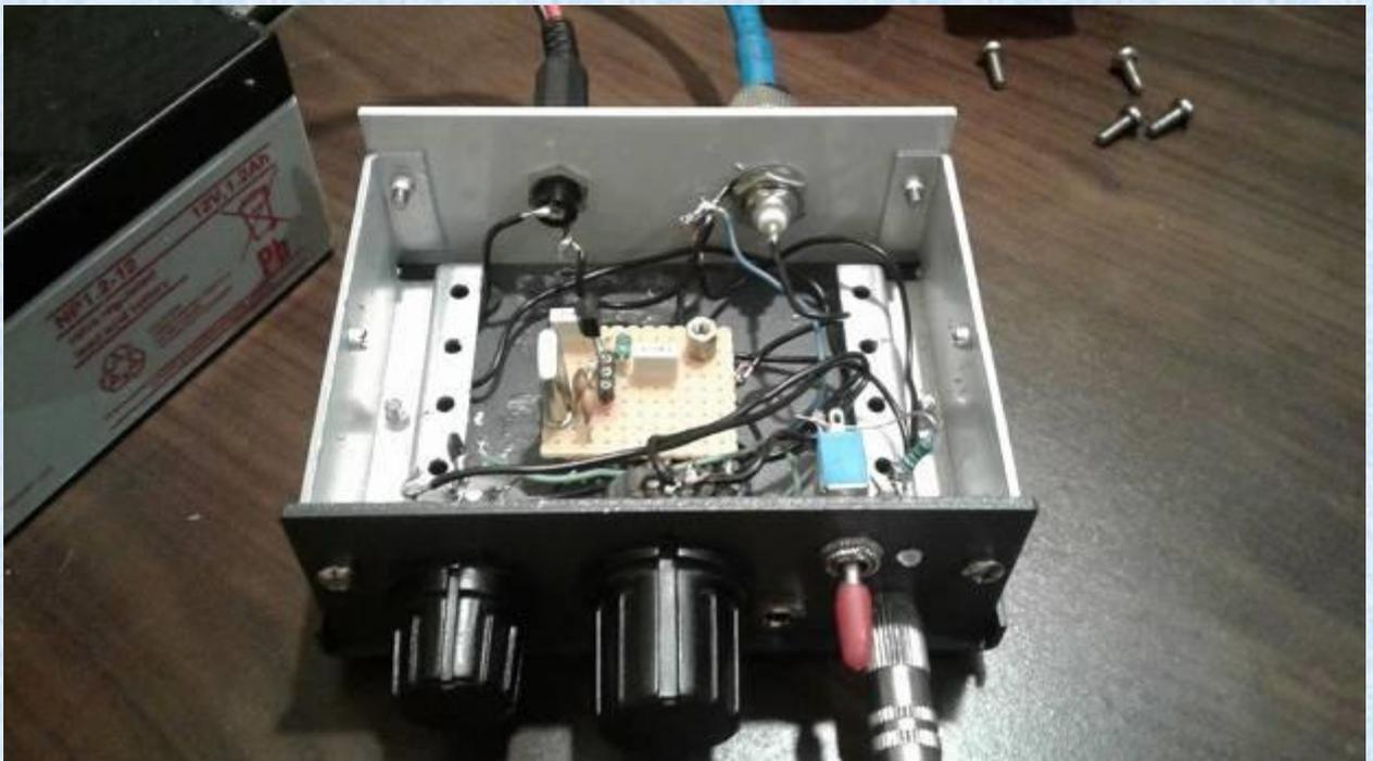
I am using the magnetic headphones. Series capacitor is needed when piezo headphones are used. With magnetic the resistor is needed, what in this case the magnetic headphones resistance replaces as required to start of the oscillation. For this R3 variable resistor is replaced with 47 kOm resistor in the trcvr I am currently using.
